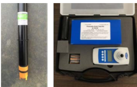
Figure 7 Commercially Available PAA Probes and Test Kits (Reprinted with permission from PeroxyChem).
