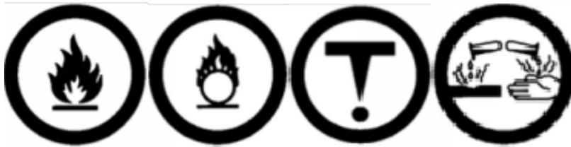
Figure 8 Workplace Hazardous Materials Information System (WHMIS) Symbols for PAA (Left to Right): Combustible Liquid, Oxidizing Material, Toxic Material, Corrosive Material (Reprinted with permission from PeroxyChem).
